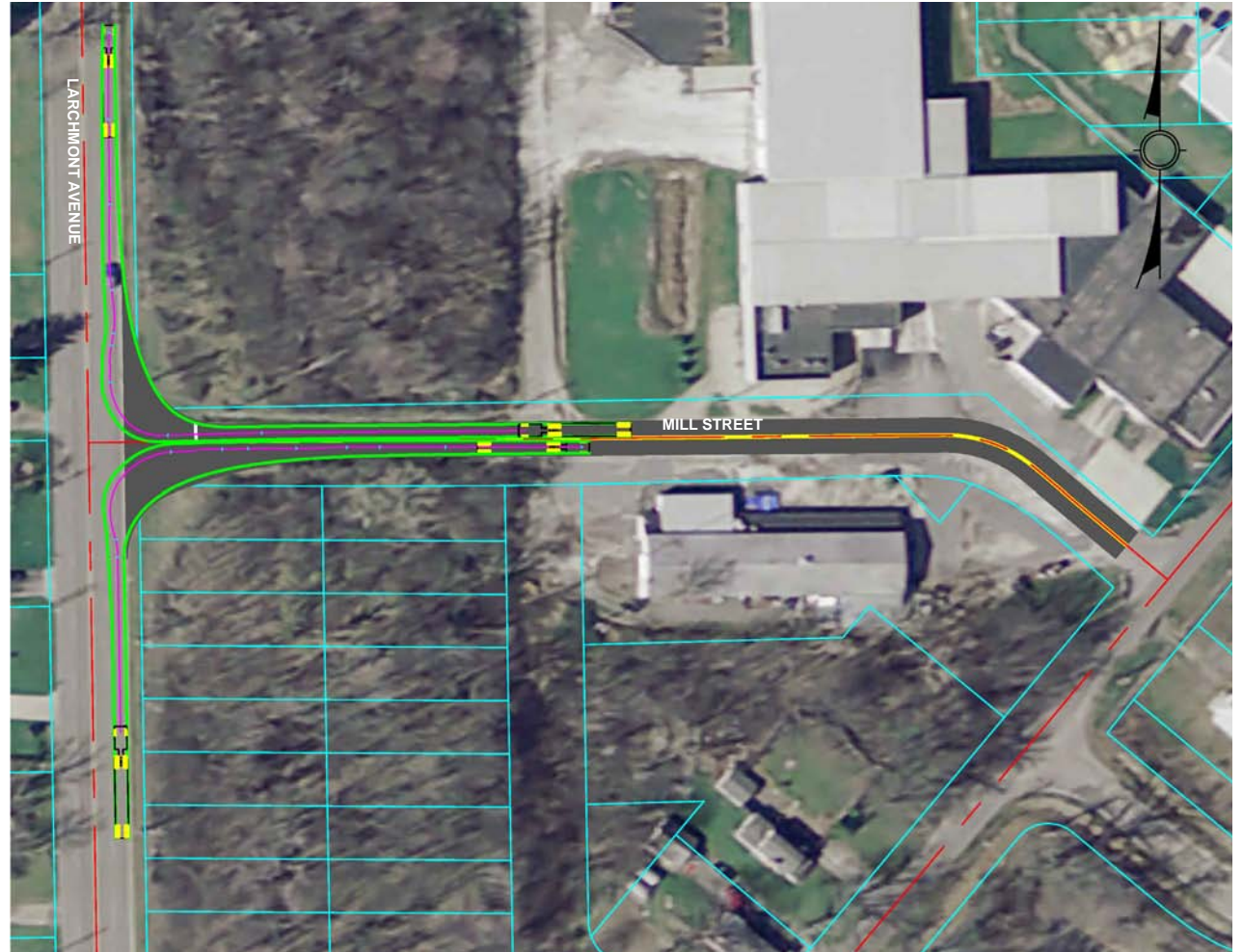
Figure 16. Mill Street Resurfacing and Larchmont Avenue Intersection Improvements
